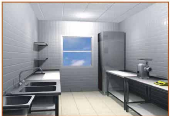
Picture 5. Preparation room for meat. Visual stimulation. Inventory: 1 – dual bowl sink; 2 – table with a chopping board; 3- table; 4 – meat chopper; 5 – shelf; 6 – refrigerator (volume – 700l); 7 – bench-type scales (up to 10kg); 8 - waste container; 9 - kitchen sink.
